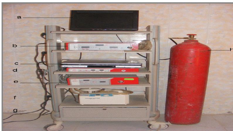
**Fig.1** : Shows the laparoscopic system which used in the experiment; a- Monitor. b- CO<sub>2</sub> insufflators. c- DVD recorder. d-Video lapro laparoscope. CO<sub>2</sub>
