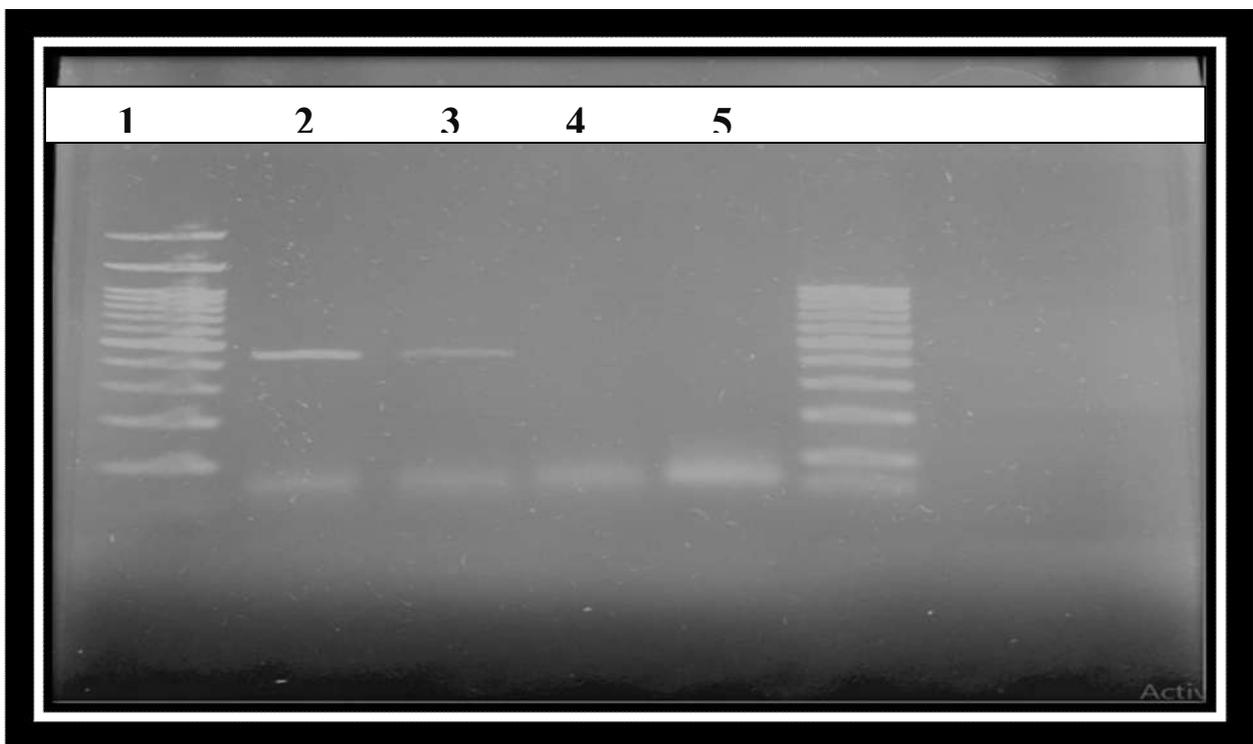
Figure 9: PCR amplification of 16S rRNA gene. Lane 1, 100 bp molecular size marker ; lane 2-5 PCR products on Agarose 1.5%.
